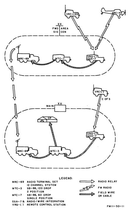
Figure 11. Type utilization of radio/wire integration stations.
