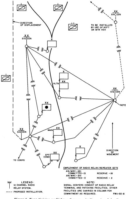
Figure 8. Type division multichannel communication network for the advance to contact.
